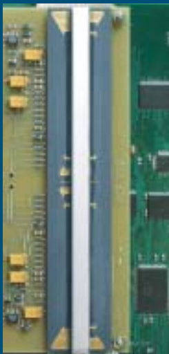
The high resolution CCD sensor with a CsI (Cesium - Iodide) scintillator screen
